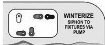
**NOTE:** When set to WINTERIZE: antifreeze will not enter the water heater or the fresh water tank. There are no dedicated water heater bypass valves.
