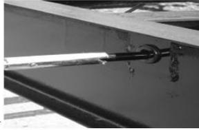
**Fig. 2-Through Frame Crank Extension w/Pin**
