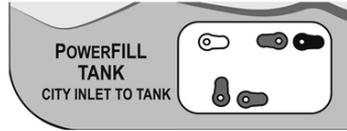
When tank is full, turn off the water source, **disconnect the hose from the water source first**, then disconnect from the utility panel.
